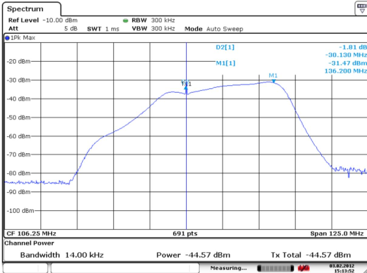
Now we get better performances with modified version and 0 dB LNA gain on FCD, but it is still a “compromise” ! We did performance measurement of the FCD receiver, it was shown poor dynamic performance and IP3 of this receiver : any signal greater than -45 dBm reduce the sensitivity by blocking receiver chain. LO leak of this converter is too high for FCD receiver. This converter can be improved but, the combination of this converter with FCD receiver is very bad.
