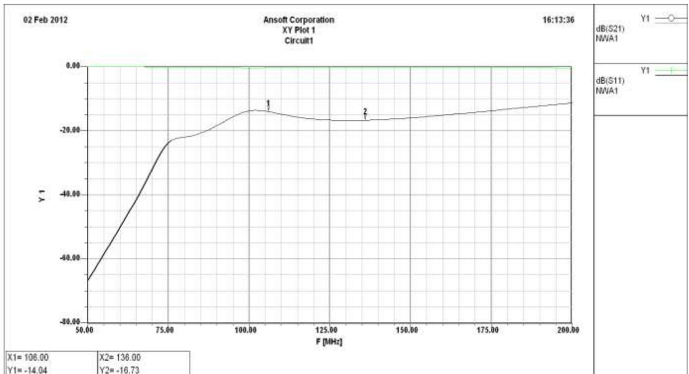
Simulation results for 1500 Ohms source impedance at input and 50 Ohms at output
