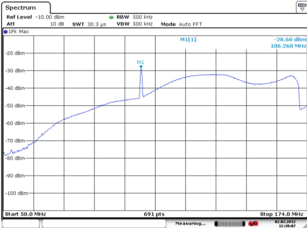
The spectrum here at converter output in max hold mode, with a swept signal of -30 dBm at converter input.
